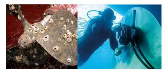
A rough propeller results in a fuel penalty for the ship. How large that penalty depends on the degree of roughness. Based on information available, it can be
