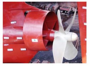
the propeller, which is again an improvement in the propeller's working condition. The duct itself creates a forward directed thrust due to its foil section shape. Becker Marine Systems delivers each Becker Mewis Duct individually adjusted for the actual hull form and propeller after a thorough design phase using Computational Fluid Dynamic (CFD) computations.
