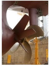
After conducting a sea trial of this vessel with this energy saving device, significant improvement in performance has measured. Indeed it accelerated Vessel's speed performance by 0.2 knots and reduced fuel consumption by 4%.
