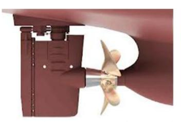
and, therefore, emissions. With Promas Lite these improvements can be maximised, as the propeller and rudder are treated as a complete system which can lead to further increases in efficiency which parallel will lead to improved manoeuvrability for only a
