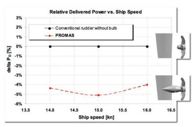
Promas Lite integrates the propeller and the rudder into a single system. Behind a normal propeller hub there is a strong low pressure vortex (hub vortex) that acts on the propeller hub, increasing drag and reducing propeller thrust. A special hubcap is fitted to the propeller which stream-lines the flow onto a bulb that is added to the rudder, effectively reducing flow separation immediately after the propeller. The result is an increase in propeller thrust, as previously
